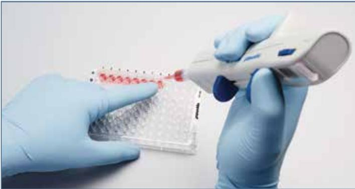
**Efficient plate work**—fill an entire 96-well plate with master mix or reagents from a single aspiration, dispense volumes as little as 1  $\mu\text{L}$
