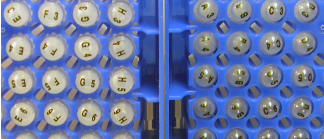
Side-by-side comparison of flat-bottom alphanumeric tubes (left) with round-bottom tubes (right).
