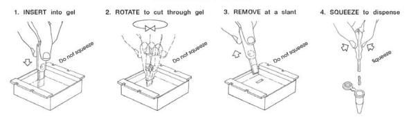
In accordance with good laboratory practice, use the x-tracta tool once, then discard it to prevent cross-contamination. Note: Do not squeeze the bulb until step 4. At step 4, use a quick snap-action squeeze to release the gel.
